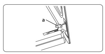
**3.** Close the door until it almost reaches the fully closed position and remove the door by pulling it towards you.
