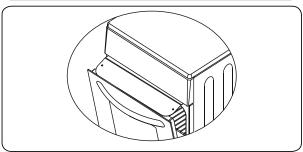
Hold the heat shield with the warnings facing upwards. There are two small slots on the right and left side of the rear edge of the shield, as shown in the figure.
