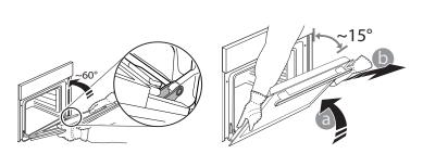
3. Refit the door by moving it towards the oven, aligning the hooks of the hinges with their seating and securing the upper part onto its seating.
