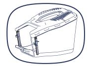
iii. Lift up the rear flap before assemble the grass bag.Hang the collection bag on the mower.
