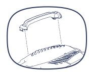
ii. Place the metal frame inside the grass collection bag. Make sure that these clips are fully secured to the metal frame.
