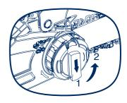
2. While holding the bar, adjust the chain tension by turning the chain tension adjust wheel (B) until the chain engages in the bar channel.
