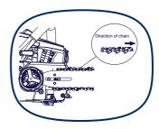
4. Adjust the tension to ensure that there is not too much slack in the chain. Make sure the tensioner pin (B) is located in the assembly hole (A) on the bar. Pay attention to the correct direction of the saw chain. Compare with the picture near the chain sprocket and the picture on the bar.
