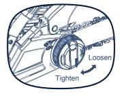
3. Tighten bar knob securely (clockwise). Hand tighten only!
