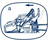
8. After engine starts, allow the saw to run and warm up in this position for 30 seconds.
