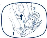
6. Push the choke control (A) in to disengage. (Failure to do this may cause the engine to flood).
