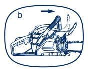
3. Press and release the primer bulb (B) 10 times.
