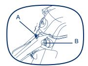
4. Pull the choke control (A) out to engage.
