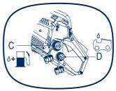
Clean surface around fuel cap to prevent contamination. Loosen fuel cap slowly. Rest the cap on a clean surface. Carefully pour fuel into the tank. Avoid spillage. Prior to fastening the fuel cap, clean and inspect the seal located inside the fuel cap. Immediately replace fuel cap and hand tighten. Wipe up any fuel spillage.
