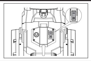
Press the switch marked "1" to start and marked "0" to stop the motor.
