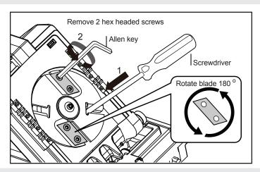
2. Since the blade is two side sharp for cutting, so could use both sides; Lock the blade disc using screwdriver or similar tools. Remove the blade by Allen key and rotate it through 180 degrees then fit the blade to the blade disc ensuring that the ground cutting edge is facing downwards; Fix the metal frame back with screws.
