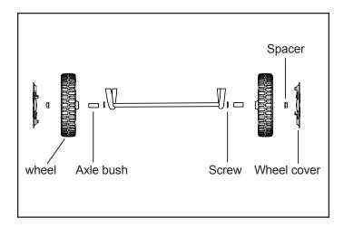
Step2. Mount the wheel in the same order illustrated, fasten nut by the provided spanner ensure the nut is not too tight.
