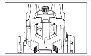
3. Close top feed, make sure knob fasten in proper position.
