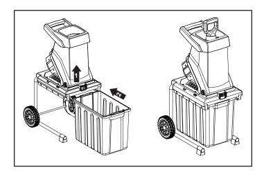
Step 4 Lift up the button, push the collection box to end of the track, and make sure the box has been locked.
