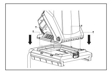
Step3. Place the motor unit on the chassis, Secure the unit with 4 screws.
