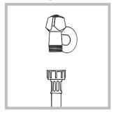
1. Connect the supply pipe by screwing it to a cold water tap using a 3/4 gas threaded connection (see
