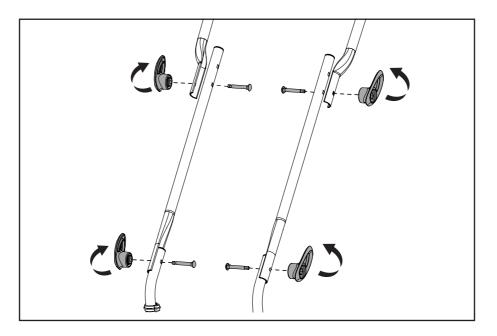
• Attach the Middle handle bar to the lower handle bar using bolts and wingknobs.
