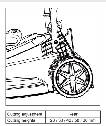
• When cutting longer grass always raise the cutting height and cut the grass in 2 or more passes by lowering the cutting height gradually at each pass, never cutting the grass by more than half its height.
