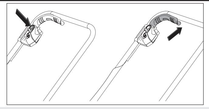
To switch on, press the safety lock-off button on the handle, then activate the start/stop switch lever. Release the lock-off button.
