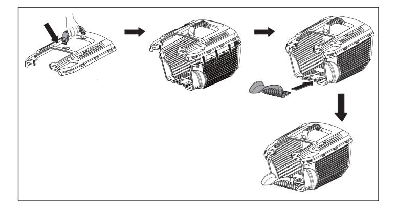
• Push fit the grassbox upper on to the grassbox lower. Start with the clips at the front and work your way to the back of the grassbox. Insert the grassbox handle into the grassbox upper. Slide the tongue on to the front of the grassbox lower.
