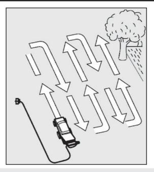
• Place the mains lead in loops on the ground near the wall socket. Mow away from the socket and cable and ensure that the mains lead is always on the section of lawn that you have already mowed so that you do not run over the mains lead with the mower. The blades can cause damage to the power cord if contact is made and risk electrocution.
