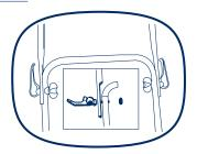
iv. Ensure the rope guide is on the right side, when you stand behind the mower. Pull start/stop bar and gently pull the starter handle. Hook it around the guide rope.
