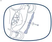
v Check the washer is still slightly domed to keep the pressure on the bold to stop it unwinding, keeping the blade firmly secure. Replace the washer (right way round!) and bolts. Note: If washer has lost its dome and become flat it must be replaced.
