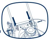
ii. Fix the lower handle onto the deck firmly, using the lower handle fixing bolts (11) and knobs.
