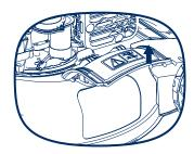
Hold the flap opening, hook the side discharge chute onto the mower and release the safety flap.
