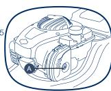
Pressing the primer button too many times could cause the engine to flood.
