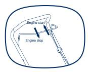
iv. With right hand, slowly but firmly pull the starter handle and rope from the pull cord guide until you feel resistance, then pull briskly. If the engine fails to start after three pulls, repeat the start process. When the engine starts, return the starter rope to the pull cord guide gently.
