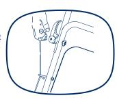
v. Release the stop/start bar to stop the machine.
