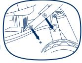
ii. Fix the lower handle onto the deck firmly, using the handle fixing bolts (11) and spanner (13) supplied.
