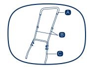
iii. Position the complete assembled handle over the studs of both sides on the rear of mower frame.
