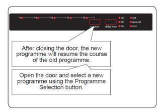
NOTE: Open the door slightly at first to stop a programme before it is complete in order to avoid water spillage.
