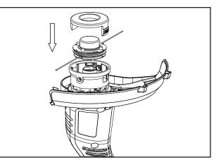
NOTE: Before replace the spool, make sure the mains plug is disconnected from the unit.
