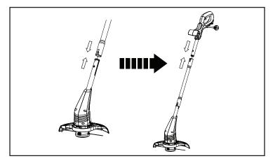
• Assemble the housing into the handle and fully engaged.
