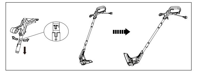
• Push the shaft forward, turn the handle to 180°, when trimming near edges and walls.
