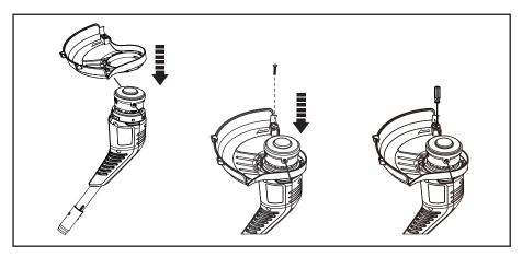
• Place the guard onto the tool as shown, secure the guard with screws.
