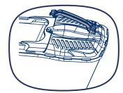
ii. Place the metal frame inside the grass collection bag. Make sure that these clips are fully secured to the metal frame.
