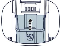
ii. Lock the collection box by rotating the safety switch to "lock" Position.
