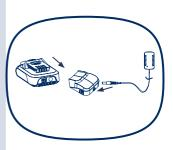
This product comes with a lithium ion battery pack. Lithium lon batteries don't lose charge when not in use, and don't lose charging capacity overtime. Never the less it is best practice to charge the battery when empty or insufficient to do the job.
