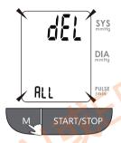
Note: To exit out of delete mode without deleting any records, press "START/STOP" button.
