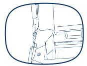
NOTE! Make sure the front plate(A) is on the bar above front roller.
