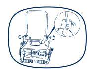
NOTE! Make sure that the cable hooks are at the back side of the machine.
