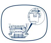
ii. Release the locking knobs and fold the handle down.
