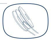
ii. Wind the line following the directional arrows on the spool housing and hook the two ends into the side grooves.
