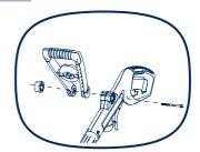
iii. Insert the bolt from the right through the opening. Ensure that the bolt head sits properly in the recessed shape in the support then tighten the knob.
