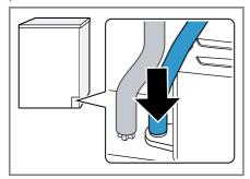
**4.** Insert the water outlet hose into the hose guide.
