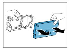
Ensure that you do not deform or damage the filter mat.
