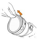
Grasp the tab on the filter and pull to remove.
