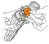
Pull to remove the brush bar location plate. Remove the belt, if the belt isn't broken rotate the cogs anticlockwise and slide the belt off the large cog first.
