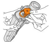
Pull to remove the brushbar location plate. Remove the belt.
