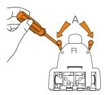
Using a crosshead screwdriver, remove the 2 screws (A) to clean the TurboTool
