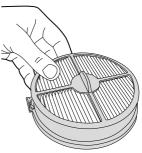
Check the post-motor filter for discolouration.
