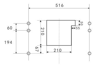
3) Install the adjusted board on the bottom of the hood in order to keep out the gap between the hood back and the cupboard.
