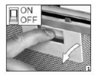
1) Remove the metal filters by pulling down the handle and pulling them away from the cooker hood. This will allow you access to the motor.
