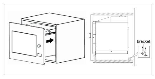
5. Open the door, fix the oven to the cabinet with Screw B, at the installation hole. Then fix the Trim-kit plastic cover to the installation hole.
