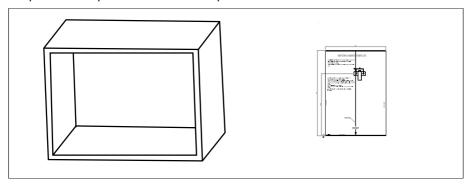
2. Make the marks on the bottom plane of cabinet according to marks "d" of of the template
