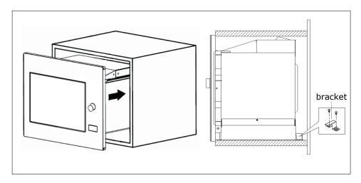
5. Open the door, fix the oven to the cabinet with Screw B, at the installation hole. Then fix the Trim-kit plastic cover to the installation hole.
