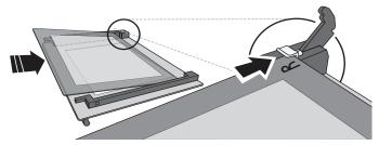
**4.** Refit the upper edge: A click will indicate correct positioning. Make sure the seal is secure before refitting the door.
