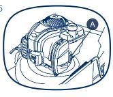
Pressing the primer button too many times could cause the engine to flood.
