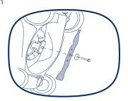
v Check the washer is still slightly domed to keep the pressure on the bold to stop it unwinding, keeping the blade firmly secure. Replace the washer (right way round!) and bolts. Note: If washer has lost its dome and become flat it must be replaced.
