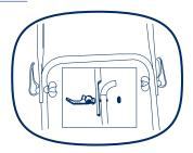
iv. Ensure the rope guide is on the right side, when you stand behind the mower. Pull on/off lever and gently pull the rope. Hook it around the guide rope.
