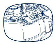
Hold the flap opening, hook the side discharge chute onto the mower and release the safety flap.
