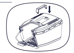
ii. Place the metal frame inside the grass collection bag, Make sure that these clips are fully secured to the metal frame.
