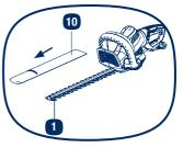
**NOTE:** Always attach the blade sheath (10) when the product is not in use, for storage and transportation.
