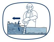
vii. Cut in a number of stages if the area being cut is particularly long to achieve a better result; smaller trimmings will allow for easy composting.
