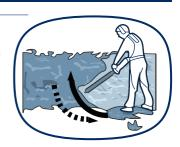
vi. After cutting the sides proceed to the top. Try to keep the cutting device angled at approximately 15° to the cutting surface.
