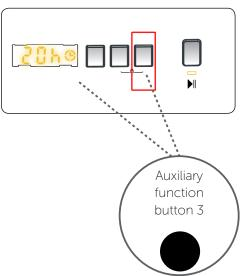
You can use this auxiliary function to delay the start time of the washing cycle for 1 to 23 hours.
