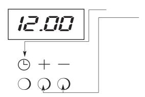
Step 3 Press the "D" button and then press either the "+" or "-" buttons to set the correct time of day.
