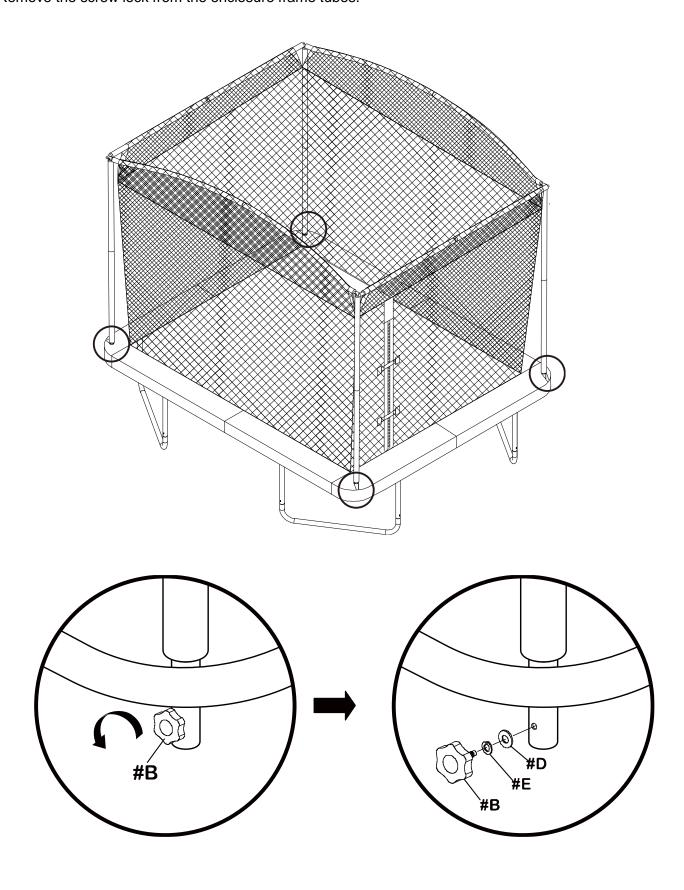
Life up the enclosure frame tubes on one side and place it onto the trampoline. Repeat the same on the other side
