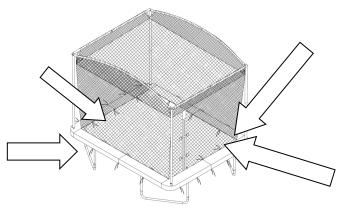
**Inspect prior to use** – check that the legs are properly attached and stable on the ground; no loose springs; mat and enclosure net are in proper place and in good condition with no tears.
