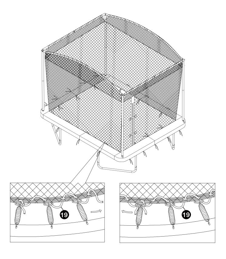
Secure the frame pad, Tie the inner straps to the triangle rings and the outer straps to the frame tubes.
