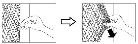
If it produces any tear or cracking or ripping sound, then the net is unsafe and MUST be taken down immediately. STOP USING THE TRAMPOLINE ENCLOSURE IF YOU FIND ANY SIGNS OF WEAR OR TEARING ON THE NETTING.
