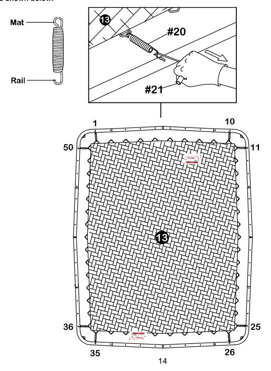
Attach springs to the middle of the frame as shown.
