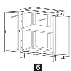
NB: For improved stability, the product should be affixed to the wall using suitable wall plugs. See reverse the product should be affixed
