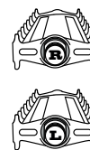
Pedals x 2 (make sure you have an 'L' and an 'R' as shown)
