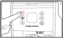
After setting is complete, the machine will beep and display the selected time for 3 seconds before switching back to the current time. To cancel this program, press the Program/Clock Button (11) again so the 'PROGRAM' icon disappears.
