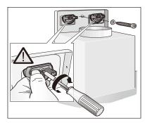
Note: The wall fixings supplied may not be suitable for all wall types, and therefore it is the responsibility of the installer to ensure the wall fixings are appropriate for the surface that the Hood/Flue is being attached to
