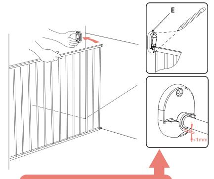
Locate the 2 holes position before (E) to be amounted on the wall.
