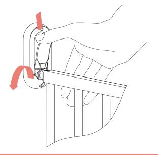
One-handed use, press down the button and lift the gate for two way opening.
