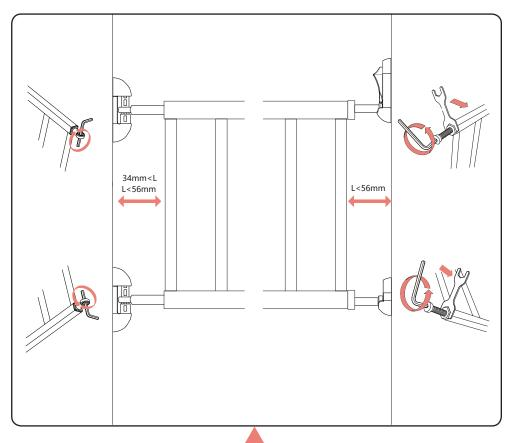
Use the tools provided to adjust bolts (I) and (J) to make the gate width to fit the door properly as below safety requirement: Caution: To ensure that this distance between each side of the gate and the wall is less than 56mm. Meanwhile, the distance between the fixed side of the gate and wall must be more than 34mm.
