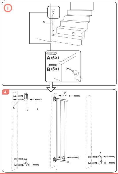
Drill 5 mm hole for the 6 marked positions, then put wall plugs (A), and use screw (B) to fix component (C) and (F).
