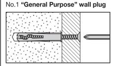
Generally aerated blocks should not be used to support heavy loads, use a specialist fitting in this case. For light loads, general purpose wall plugs can be used.
