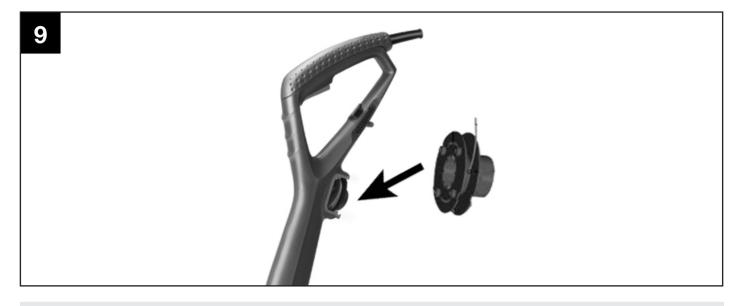
A spare cutting line spool can be stored in the recess below the rear handle. If you store your spare spool here it will always be ready to hand when the line on the spool being used runs out.
