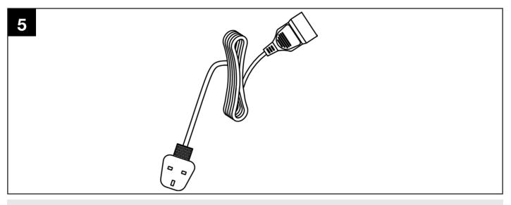
Connect the extension lead socket to the plug on the mower. Hook the cord of the extension lead through the cord retainer. This helps to prevent accidental disconnection during usage.
