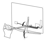
Do not use a sharp object when you detached the cable cover. This could damage the cable or the cabinet. It may also cause personal harm. (Depending on model)
