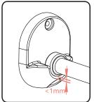
Locate the 2 holes position before (E) to be amounted on the wall.
