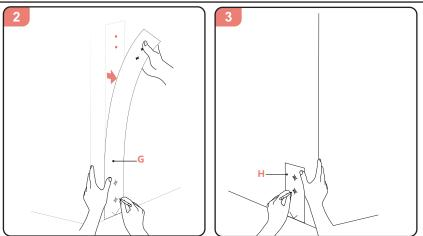
Cut the installation template following the dotted line. Stick the longer one (G) in one side of wall and shorter one (H) to the directly opposite wall.
