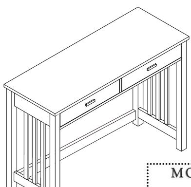
"It is recommend to use a PVA glue bought from a reputable DIY store to secure the components E when assembling the product"
