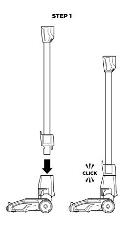
1 Insert the wand into the motorized floor nozzle connector until you hear a click.
