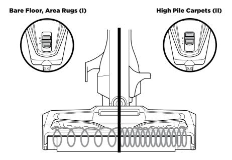
The Shark® Rocket™ Complete with DuoClean™ has a 2-speed power slider switch on the handle. Slide the power switch to appropriate speed setting (I or II) and start cleaning.
