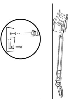
2 Use the wall mount that is included. Drill two 5/16" holes into the wall and insert the provided plastic anchors into the holes. Using a Phillips-head screwdriver, screw the wall mount into the plastic anchors. Hook the catch on the bottom of the handheld vacuum onto wall mount.
