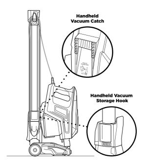
1 Press the Wand Release button on the top of the wand to release the handheld vacuum. There is a catch on the bottom of the handheld vacuum. Hang it from the hook located on the bottom portion of the wand. Wrap the cord around the two cord hooks.
