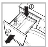
To remove the drawer, press lever (1) and pull the drawer outwards (2) (see figure). Wash it under running
