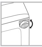
2. If the floor is not perfectly level, compensate for any unevenness by tightening or loosening the adjustable front feet (see figure); the angle of inclination, measured in relation to the worktop, must
