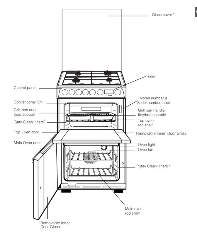
NOTE: To keep the controls cool when the appliance is used, a flow of air may be blown from beneath the control panel. If the appliance is still warm, this cooling fan will run on when all controls have been turned off. This is normal and is not a fault.
