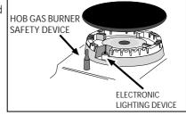
you must hold the control knob in for about 3-7 seconds after the burner has been lighted to allow the gas to pass until the safety thermocouple has heated.
