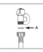
1. Insert seal A into the end of the inlet hose and screw the latter onto a cold water tap with a 3/4 gas threaded mouth (see figure). Before making the connection, allow the water to run freely until it is perfectly clear.
