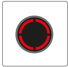
If the brush bar jams during use, the AirRam K9 will stop and the LEDs will appear red. You will need to remove and clean the brush bar (see page 11).
