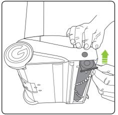
Re-insert the brush bar, starting by the end furthest away from the button. Then line up and push the brush bar into the AirRam K9 until it clicks into place.
