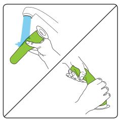
Wash the filter under a tap. Squeeze out any excess water then let it **dry completely** before reinserting into the AirRam. Recommended water temp 40°C do not use detergent. **Never put bin back** without filter inside. You could damage the motor.
