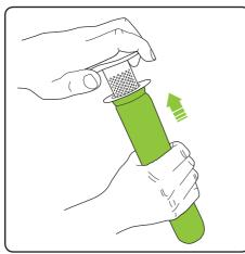
Slide the filter onto the inner shroud.
