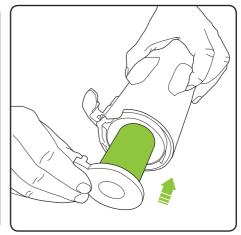
Slide the filter and inner shroud into the filter housing.
