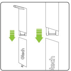
Fit the two components of the lower handle together in the orientation shown in the image above. They will only fit together one way. The components will click into place and will remain permanently fixed.
