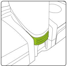
The green locking clip, when correctly fitted, will click and and hold the lower handle in place. Should the handle assembly need to be removed the clip can be pulled out to unlock the lower handle.
