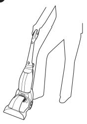
For best results apply the solution on the forward stroke (press trigger) and recover the solution on the backward stroke (release
