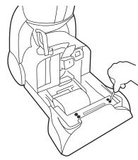
Unscrew 2 retaining screws located on the underside of the detergent nozzle. Remove the brushbar from the nozzle.
