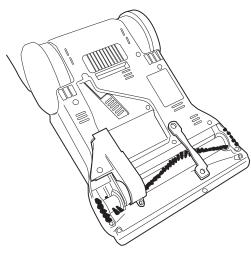
Replace the agitator by looping the belt round the agitator making sure it sits securely in the belt channel.
