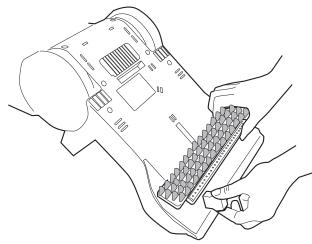
Replace the brush bar and attach to the nozzle. Attach the alignment brackets and assemble to the cleaner.
