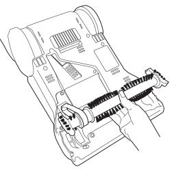
Reassemble the agitator assembly to the cleaner ensuring the agitator can rotate freely.
