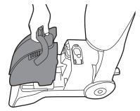
Turn the tank cap anti-clockwise to open.
