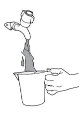
Pour the solution into the clean water thank. Do not exceed the max fill line. Replace the cap and return the clean water tank to the cleaner.
