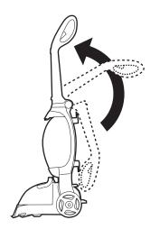
Once the handle has been lowered lift the carry handle to allow the cleaner to be carried from room to room.
