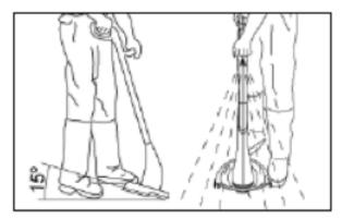
4. If the grass is very long cut in stages rather than trying to cut in one ago. Do not overload your trimmer, take small cuts this will keep machine operating at high speed and will greatly improve cutting efficiency.
