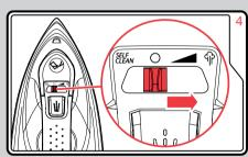
Vary the steam output using the variable steam switch (1), as shown above.
