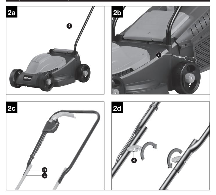
**2a-2b.** Fit a bottom handle into the opening provided for it and secure it as shown in Fig. 2b with a screw 7. Proceed in the same way on the other side.
