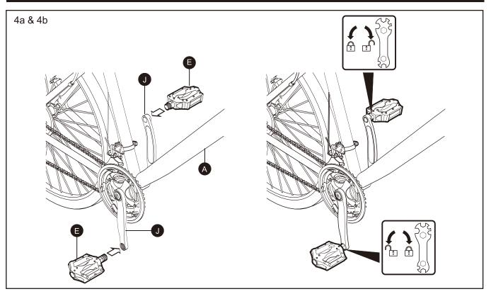
NOTE NOTE! The pedals and crank arms I have colour coded stickers to indicate which pedal matches which crank arm I.
