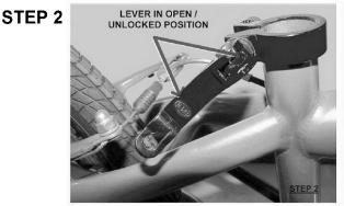
THE QUICK RELEASE CLAMP IS MARKED OPEN & CLOSED. WHEN IN OPEN POSITION, SEAT POST CAN BE INSERTED INTO THE FRAME TO THE DESIRED HEIGHT POSITION
