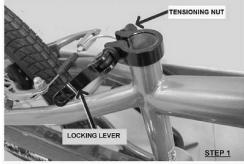
YOUR BICYCLE WILL HAVE A QUICK RELEASE CLAMP INSTALLED FROM FACTORY
